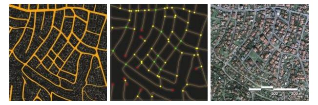
Figure 5. Gazi (Zübeyde Hanım): urban fabric and road network. Note: The picture on the left shows the coverage ratio; the middle picture, connecting nodes and road branches.
